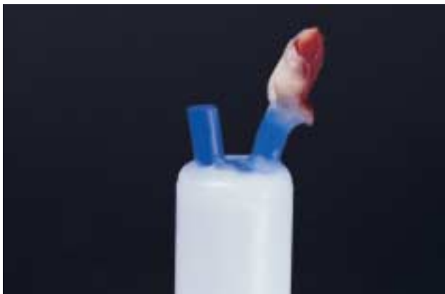
The attachment points of the sprue to the object and sprue former must be rounded and smooth. Avoid sharp edges.
