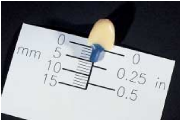
Length of the sprues: 3 mm to 8 mm
