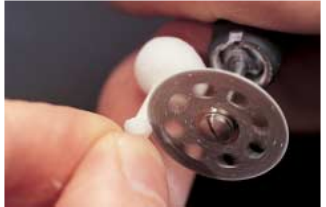
Use a fine diamond disk to cut the sprues.
