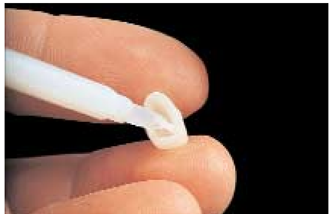
Coat the inner surfaces of the ceramic object with IPS Empress Die Material Isolating Liquid.
