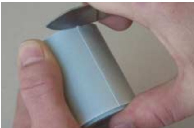
The slight material overlap created by the paper ring is also removed with a plaster knife until the line is no longer visible.
