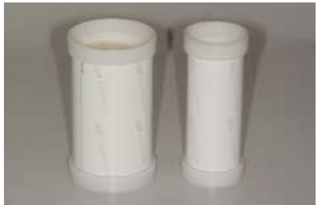
Set the paper ring on the base of the investment ring and check for correct fit. Use the ring stabilizer to stabilize the paper ring.
