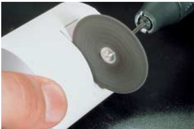
Separate the investment ring using a separating disk. This predetermined breaking point enables reliable separation of the AlOx plunger and the ceramic material.
