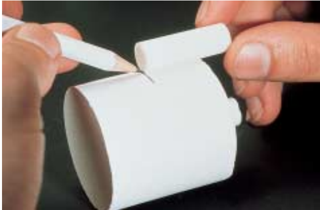
Mark the length of the AlOx plunger on the cooled investment ring.
