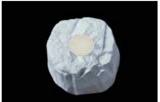
For fine divesting, only 2 bar (30 psi) pressure is applied.
