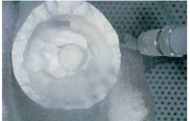
Rough divesting is carried out with glassbeads (Ivoclar Vivadent Polishing Jet Medium) at 4 bar (60 psi) pressure.
