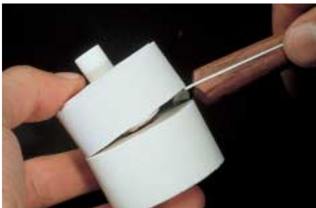
Break the investment ring at the predetermined breaking point using a plaster knife.
