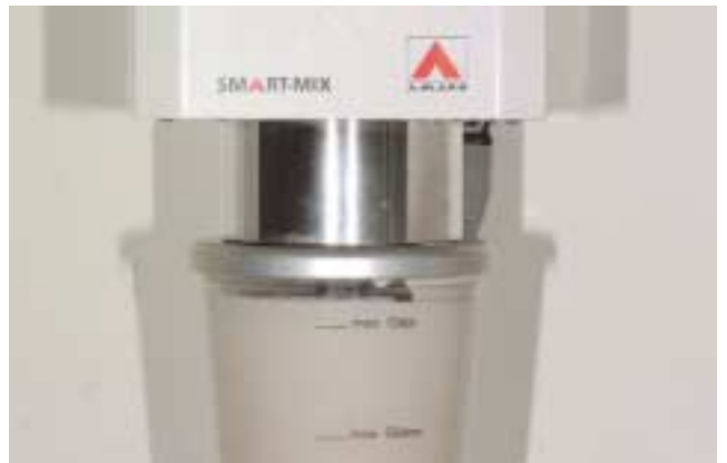
Mix IPS Empress 2 Special Investment or IPS Empress 2 Speed Investment material under vacuum. Check the vacuum.
