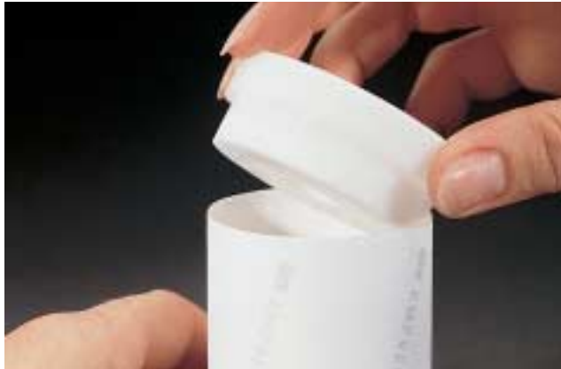
Remove the stabilizing ring and slowly place the ring gauge on the investment ring with a hinged movement.
