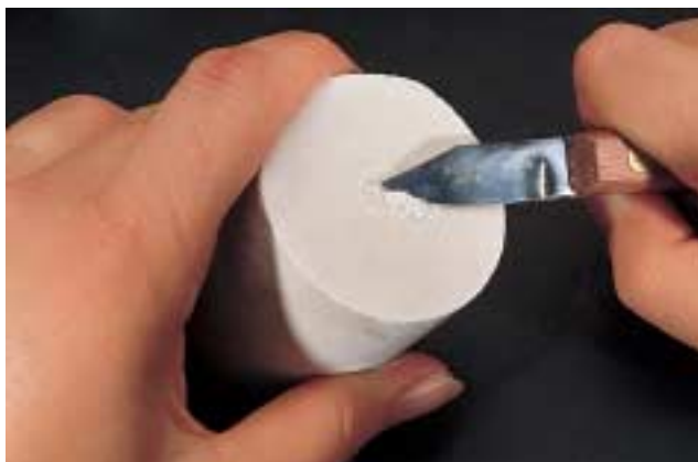
Remove rough spots on the bottom surface of the investment cylinder with a plaster knife.
