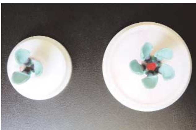
If several veneers are sprued at the same time, they should be arranged in a turbine shape.
