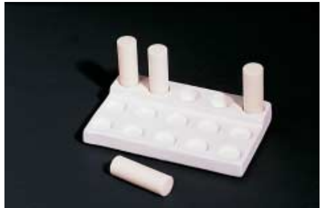
The ingot support and AIOx plungers are placed in the cold furnace.
